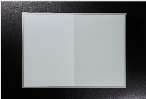
Fig. 1: Comparison of white tone by daylight: normal translucent white in signage (right); PLEXIGLAS® LED Pure White WH52 (left)
